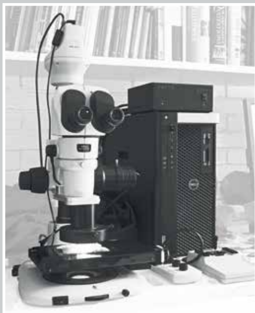
Fig 10: Richard's system, which includes the microscope, LED lighting, a motorised stage and a focus motor is an example of how a microscope can be automated for relatively little outlay.
