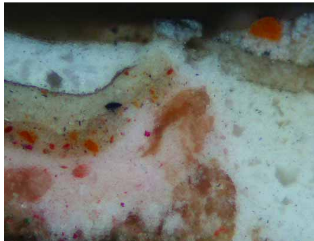
Fig. 15. St Paul's Cathedral, sample from the Whispering Gallery walls showing the original Thornhill decoration to the left and 19th Century overpaint to the right. The 19th Century overpaint fills a loss in the Thornhill paint. Later overpaint is present on the surface of the sample. Photographed in dark field reflected light at 200x magnification.
