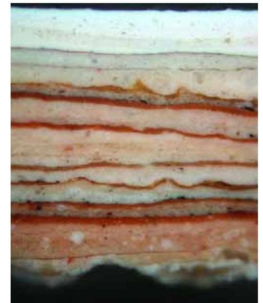
Fig. 10. St Martin-in-the-Fields Church, sample from the Apse, which shows the original gilding overlying the original paint scheme of four layers of stone colour paint. A further five gilding schemes are present, before the area is painted plain white, probably during the early 20th Century. Photographed in dark field reflected light at 200x magnification.
