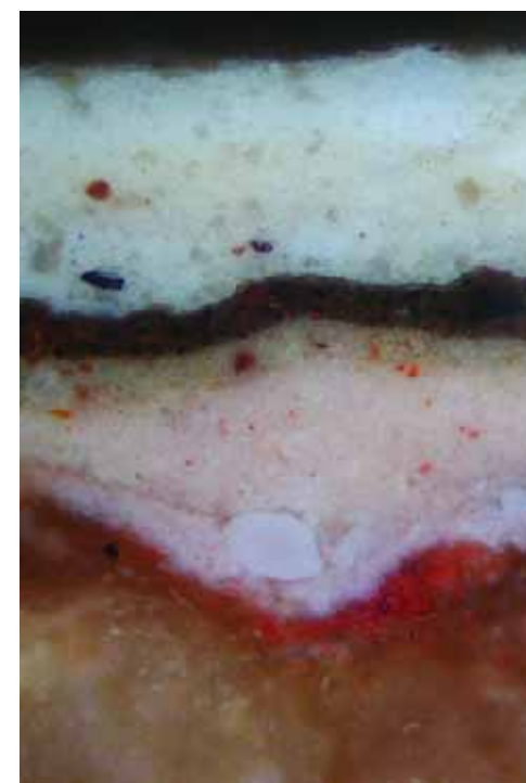
Fig. 17. St Paul's Cathedral, sample from the Whispering Gallery walls, which shows the original Thornhill decoration with a dark surface paint. When the Thornhill painting was visible this area would have represented a shadow. Photographed in dark field reflected light at 200x magnification.
