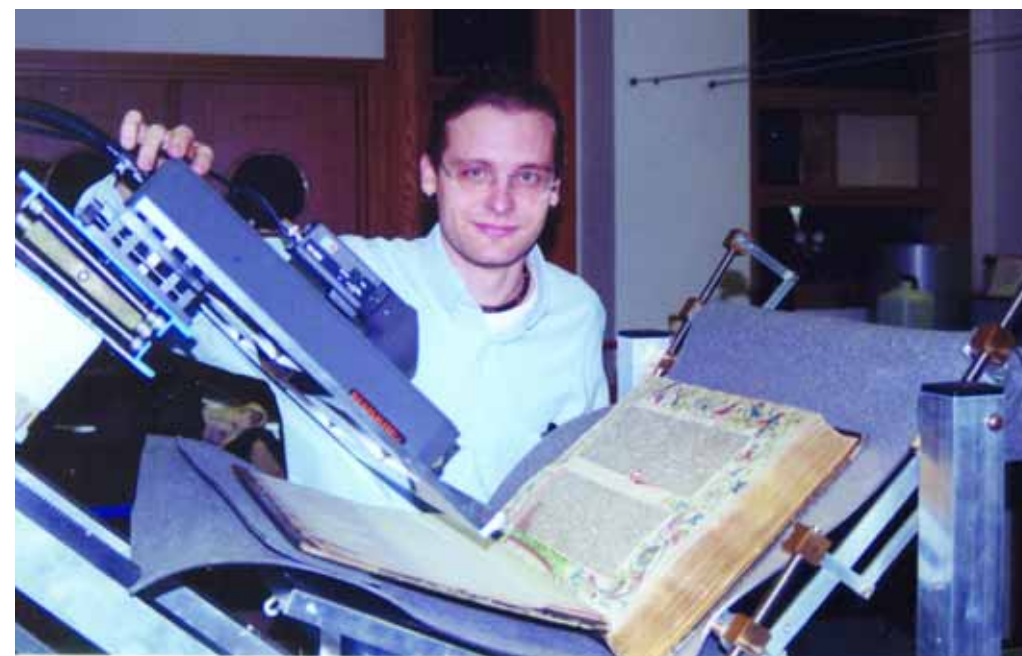
Fig. 3. Remote probe head used to deliver the laser beam onto the surface of an object which cannot be accommodated under the microscope; the probe is held on a specially constructed support which includes a book cradle. (Reproduced with permission, Elsevier Masson, Clark, 2002).
