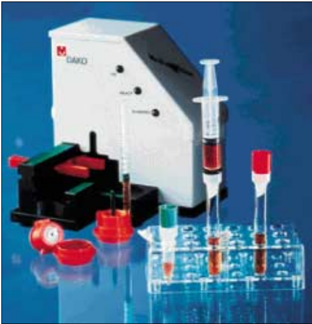
Figure 1. The MediMachine for automated tissue dissociation.
