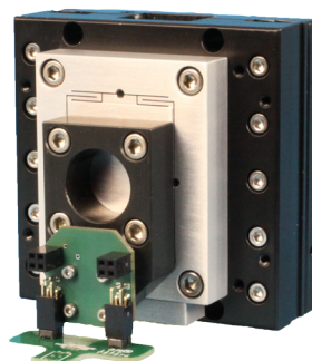
◀ A simple probe positioning configuration. This probe positioner uses an MMP1 automated positioner for the z-axis approach and a Nano-OP30 nanopositioning system for the high resolution probe positioning and feedback. The adapter for the probe mounting board is included with the MadPLL® controller.
