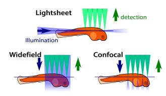
JKrieger / CC BY-SA 3.0. "LSFM: Lightsheet Fluorescence Microscopy, WF: widefield microscopy, CF: confocal microscopy." Wikimedia Commons, June 7th 2013, 20:10, https://commons.wikimedia.org/wiki/File:Lsfm\_lightsheetinsample.svg. Retrieved and modified May 1st 2019
