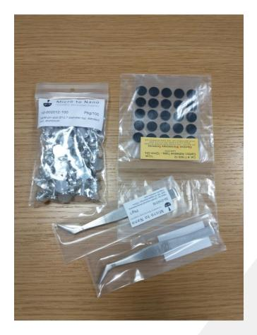
We provide stubs and self-adhesive carbon tabs to mount your samples.
