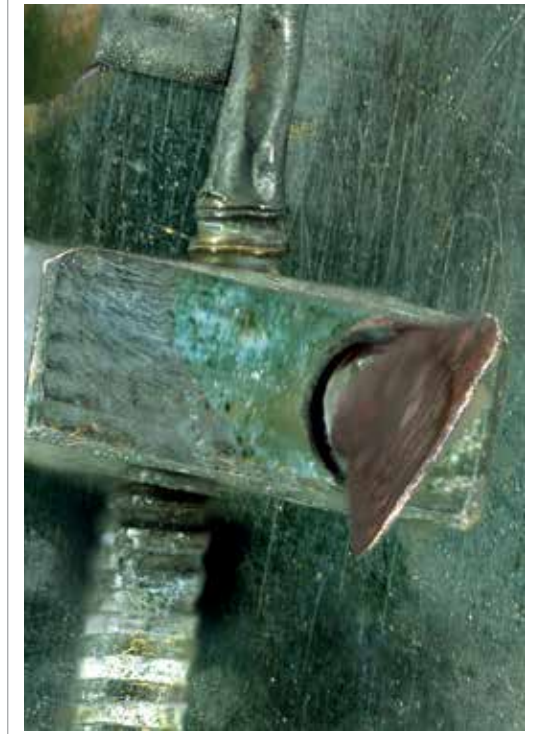
Figure 7: Care was taken to capture close-up images of the twelfth microscope with the Zuiko macro lens, and specific components (like the focussing adjustment, right) were separately photographed for superimposition. By optimising exposure and illumination levels we can maximise the detail visible. Note the canal detritus in the threads of the main screw (lower left).
