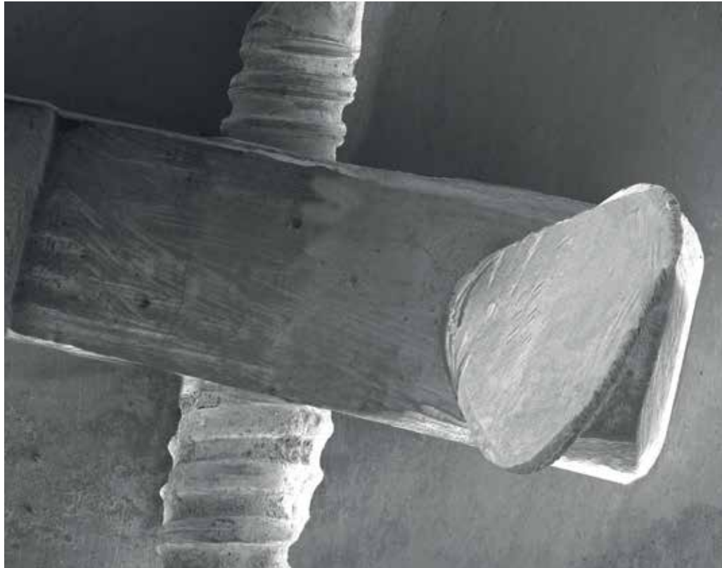
Figure 8: SEM macrography provides evidence of the hand-working of the brass, and diagnostic details of the screw threads. The apical groove along the crest of the thread and its greater diameter than the brass pin above, shows that it has been rolled. The screw threads of typical replicas are cut with a die. This approach provides far more insight than conventional photography.
