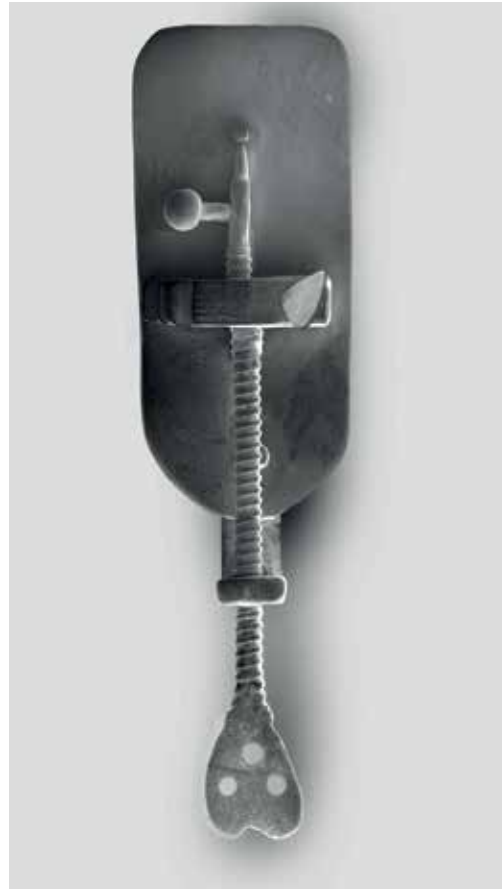
Figure 5: This SEM macrograph was assembled from 70 frames taken with the Hitachi S-3400N variable-pressure microscope at the Cavendish Laboratory, Cambridge. It correlates with the digital camera image from the Olympus E-500 camera with Zuiko Digital 35mm macro lens and assembled from 40 frames (fig 4). These images measure 27,000 pixels (2.18 cm) long.
