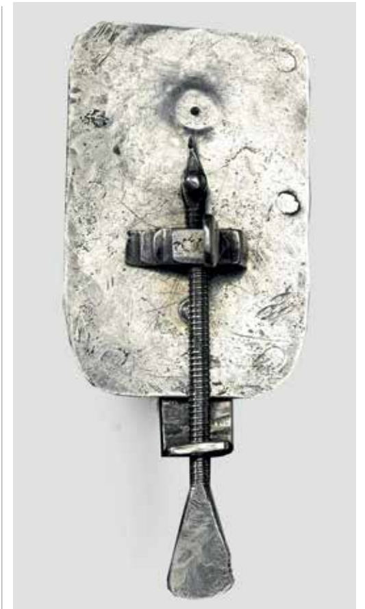
Figure 3: Hidden among doll's house toys, this silver microscope lay for years in a drawer. Occasionally it was polished. The owner brought it into a London auction house, where I was asked if it might be authentic. There is no reason to doubt its genuine nature. This is the eleventh in the Leeuwenhoek list and it encouraged me to develop objective means of establishing authenticity.
