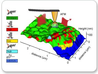
Correlative analysis of spatial map reconstructed from separate correlated AFM and chemical measurements reveal molecular orientation of vacuum-deposited PTCDA defects. *Science Advances*, 2 (10), e1601006 - E. A. Muller, et al.
