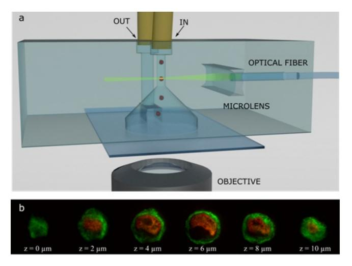
The whole device is realized using femtosecond laser micromachining, a versatile technique that allows the fabrication of 3D structures in biocompatible and inert materials like fused silica glass. The precision of the technique allowed us to shape the microchannel in order to reduce to the minimum the optical aberration in signal detection and to optimize the microlens profile, to be compatible with different excitation wavelengths.
