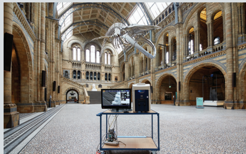
The tabletop SEM microscope at the Natural History Museum's Hintze Hall, demonstrating its portability; just a single plug socket required to get going.
