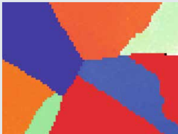
Left: Raw data of a high speed orientation map of austenitic steel (630 patterns/s, 4x4 pixel binning, 0.1 % zero solutions). Right: Enlargement of the white frame in the left image, clearly showing that indexing is as accurate along grain or phase boundaries as it is within grains.
