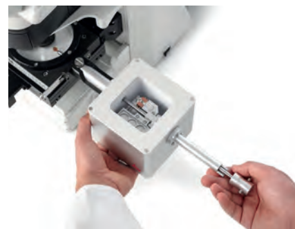
Loading of a grid cartridge into the THUNDER Imager EM Cryo CLEM using the transfer shuttle
