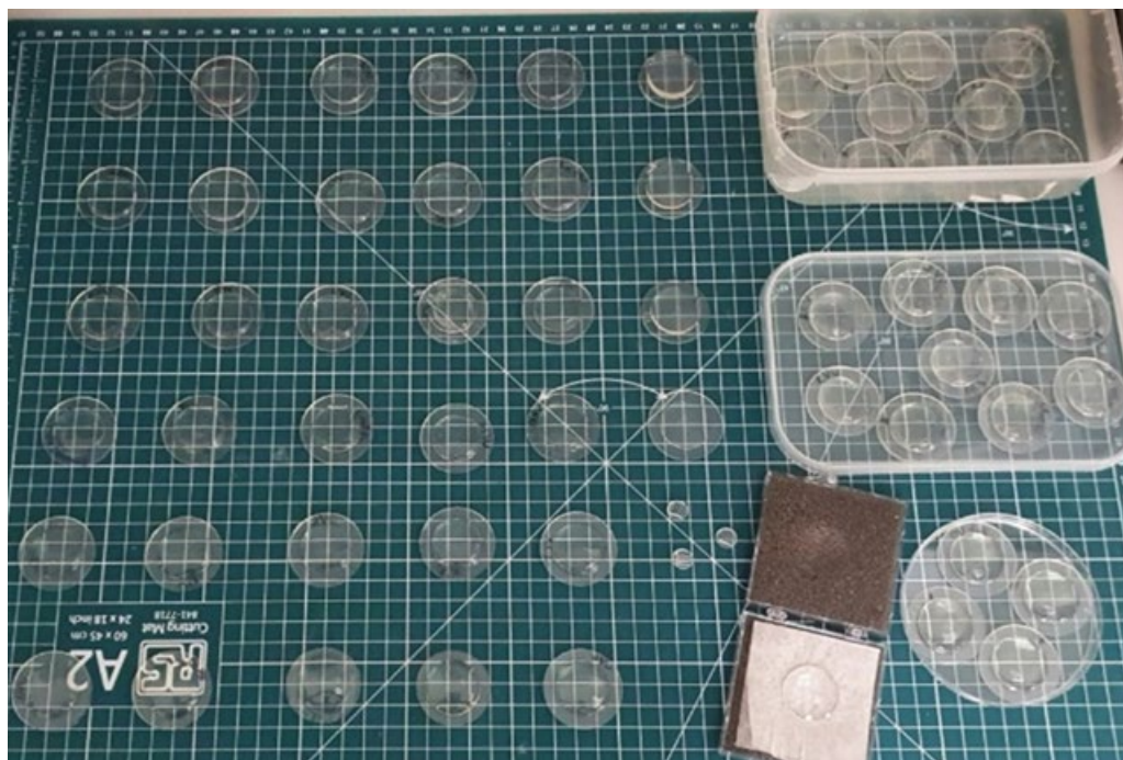
Figure 1. An overview of lenses printed during the project. Multiple lenses were printed and processed using different spin coating conditions, tested by IRM, and their surface profile characterised and compared to a glass lens of the same prescription. Each of the 3D printed lenses were printed with a thin raft surrounding the lens to ease handling, these rafts did not alter the optical parameters of the lenses.
