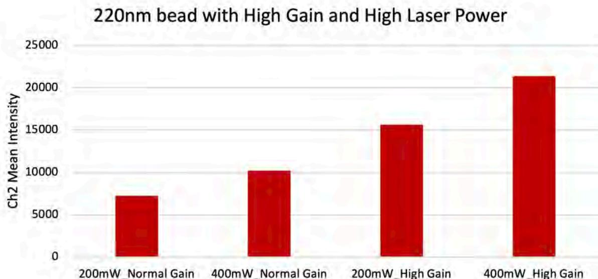
Figure 2. Increased fluorescent signal using High Gain mode and a 400mW 488nm laser on 220nm yellow SPHERO™ Nano Fluorescent particles.
