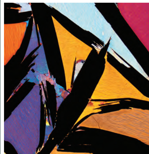
Graphite and alkali feldspars in granulite. Kerala, India. Width 3,6 mm.
