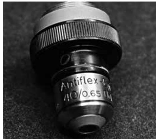
Figure 1. An early Carl Zeiss antiflex x40 objective developed for the study of the reflection of black coal. Note the low Numerical Aperture (NA) of 0.65, sufficient for reflection microscopy of dark coal
