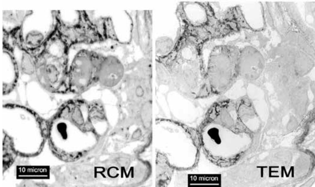
Figure 10. (Left) An image of an ultrathin section (90 nm) obtained with RCM is compared with a low magnification TEM image (right) of a sequential ultrathin section. Quite similar microscope images can be obtained
