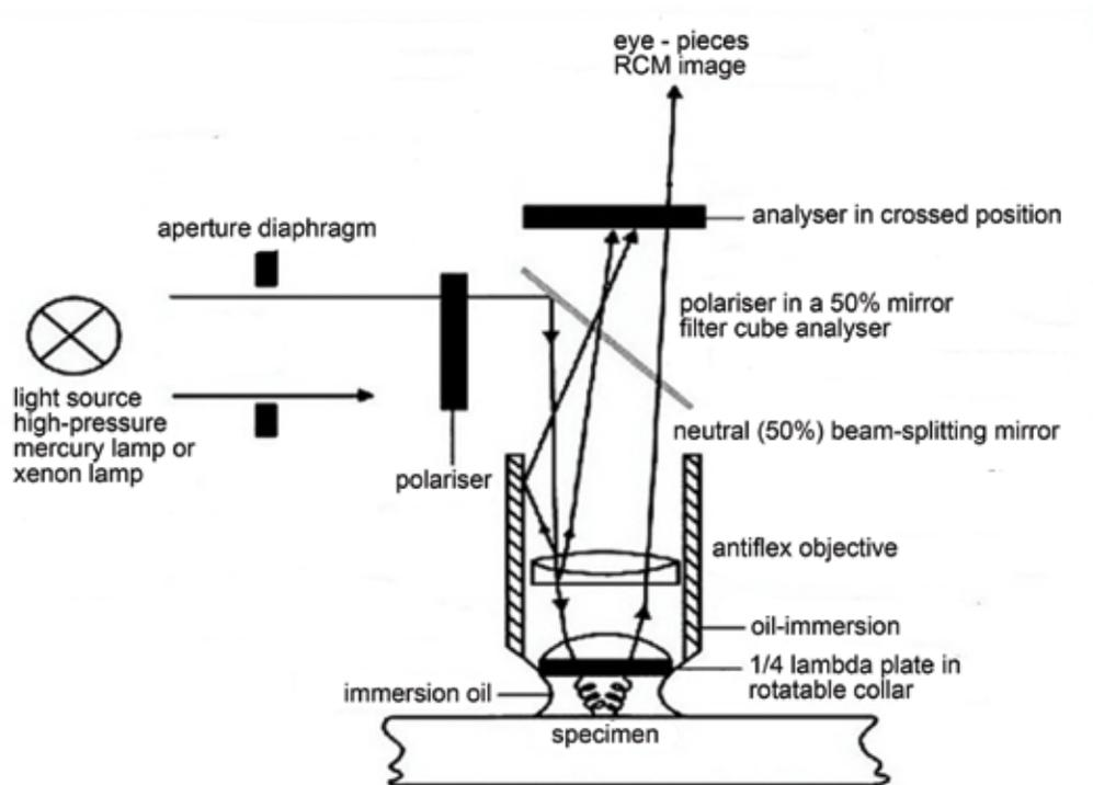
Figure 3. Light path in a reflection contrast microscope with an antiflex filter cube
