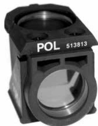
Figure 4. Filter cube for RCM, containing a polariser, a neutral (50%) beam-splitter and an analyser. This filter cube can be inserted into one of the positions of a epi-illuminator for fluorescence microscopy and will perform the antiflex functions described in Figure 3
